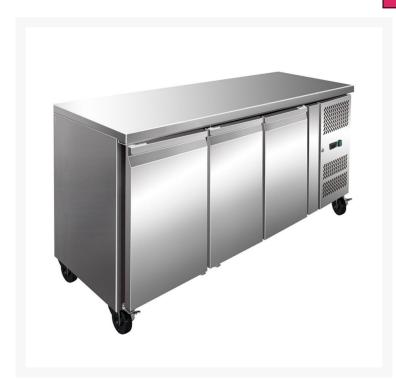
Thermaster FE3100BT S/S Three Door Bench Freezer includes stainless Steel Two Door Commercial Bench Fridge 386Litre, -18 to -22 degrees C Temp Range, one Level of Shelving Plus Floor, stainless Steel Interior & Exterior, fan-Forced Evaporator Cooling, CFC Free Refrigerant and Foam, electronic Thermostat and Digital LED Temperature Display, and auto Defrost.
