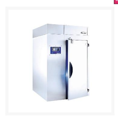
Williams Roll In WMBCF240C 1 Solid Door Blast Chiller Freezer has 1x 2/1 trolley, 240kg storage capacity, 1470mm (W) x 2350mm (D) x 2385mm (H) dimension size, 650kg of weight, 1 solid door, stainless steel finish, and R404a refrigerant gas.
