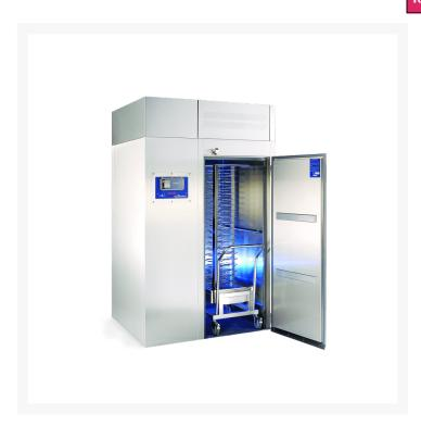
Williams Roll In WMBC200C 1 Door Combi Blast Chiller Cabinetr has 200 kg of storage capacity, 1670mm (W) x 1250mm (D) x 2295mm (H) dimension size, 650kg of weight, 1 solid door, stainless steel finish, accommodates 1/1 or 2/1 Gn combi mobile rack, and R404a refrigerant gas.
