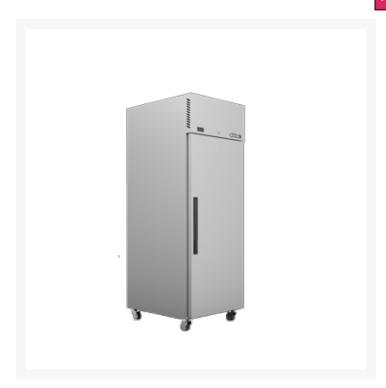
Williams Crystal RC1TSS 1 Door Bakery Stainless Retarder has 730 litres storage capacity, -5 to 3 degrees celcius temperature range, 737mm (W) x 922mm (D) x 2120mm (H) dimension size, 160 kilograms of weight, 1 solid door, stainless steel finish, and R134a refrigerant gas.
