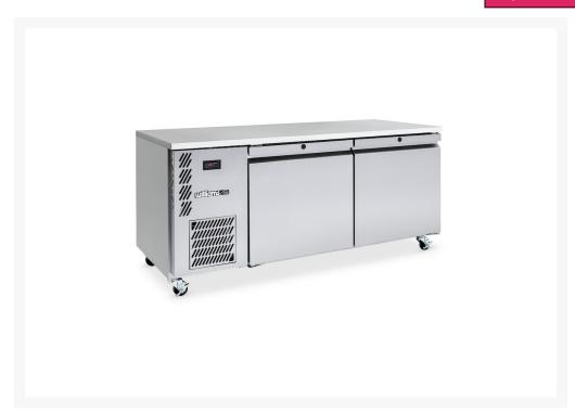
Williams Emerald LE2USS 2 Door Stainless Underbench Freezer has R404a refrigerant gas, 4 shelves, stainless steel finish, 2 solid doors, 160 kilograms weight, 1816mm (W) x 800mm (D) x 850mm (H) dimension size, -18 to -22 temperature range, and 610 litres storage capacity.
