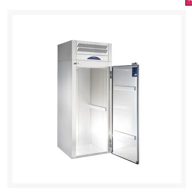
Williams Ruby HRMR1T 1 Door Stainless Steel Roll-In Fridge has a 1237 litres of storage capacity, 1 to 4 degrees celcius temperature range, dimension size of 905mm (W) x 982mm (D) x 2370mm (H), door opening height of 1776mm, 1 solid door, internal and external stainless steel finish, and R134a refrigerant gas.
