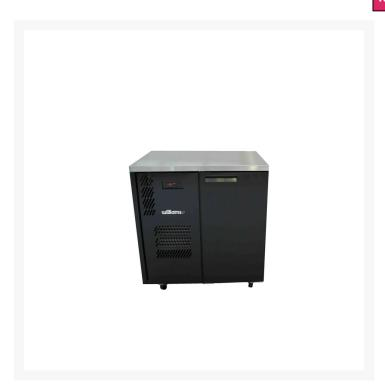
Williams Cameo HC1USB Black 1 Glass Door Fridge & Back Bars have 200 litres of storage capacity, 1 to 4 degrees celcius temperature range, dimension size of 977mm (W) x 650mm (D) x 1050mm (H), 160 kilograms in weight, 1 solid door, black finish, 2 shelves, and R134a refrigerant gas.
