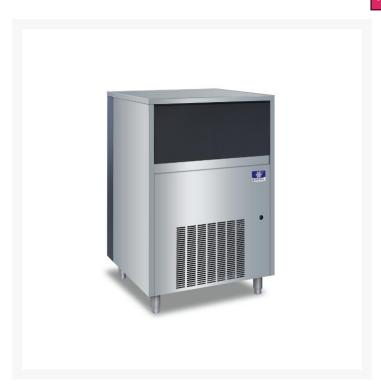
MANITOWOC-UFK0350A is an under-counter machine type that has a dimension of 738mm (L) 690mm (D) 1001mm (H), an adjustable bin legs of 114mm to 152mm, an eco-friendly refrigerant gas of R452A, the energy consumption of 4.99kWh, a bin capacity of 55kg, power supply of 220W/50/1ph, has an 1800mm power cord with no plug.
