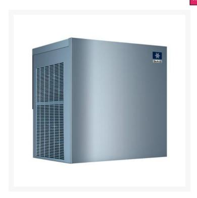
MANITOWOC-RFK0320A is an ice machine head unit, it can generate 170kg of ice a day, has a R452A refrigerant gas, 220/1ph/10A power supply, an ambient temperature range of 10 to 43 degrees centigrade, an operating temperature of 3 to 32 degrees centigrade, a dimension of 559mm (L) 600mm (D) 660mm (H), and a bin storage of 147kgs.
