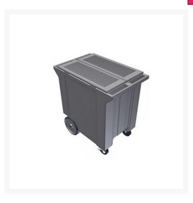
KLOPPENBERG-PCC250 is a ice transport machine type, has a 127mm front wheel castor and 254mm rear wheel castor, a storage capacity of 114kgs, a weight of 45kgs, and a dimension of 559mm (L) x 762mm (D) x 965mm (H).
