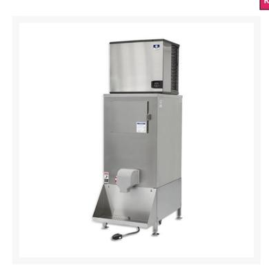
KLOPPENBERG-DISP-500T has a dimension of 762mm (L)  $\times$  1334mm (D)  $\times$  1630mm (H), a standard 240V/1ph power supply, has a adjustable stainless steel feet, has a front access single door, a safety interlock door switch that prevents operartion when the door is open and can hold up to 250kg of ice.
