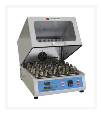
Thermoline TU-480 Economy Shaking Non-Refrigerated Incubator has an internal dimension of 450mm (W)  $\times$  390mm (D)  $\times$  370mm (H), an external dimension of 520mm (W)  $\times$  550mm (D)  $\times$  610mm (H), a swing out door type, temperature range of 5 to 70 degrees centigrade, and an orbital shaking system.
