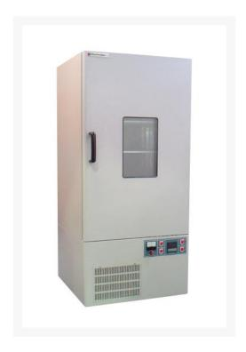
Thermoline TLM-590 Refrigerated Shaking Incubator 490L is an upright vertical cabinet type, has an internal dimension of 700mm (W) x 580mm (D) x 1100mm (H), an external dimension of 790mm (W) x 793mm (D) x 1650mm (H), a temperature range of 5 to 60 degree centigrade, an orbital shaking system, and a shaking rate of 300 RPM.
