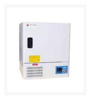
Thermoline LE-509 150 Litres Economy Refrigerated Incubator has an internal dimension of 580mm (W) x 490mm (D) x 490mm (H), the external dimension of 690mm (W) x 690mm (D) x 890mm (H), temperature range of 5 to 60 degrees centigrade, 150 litres storage capacity, and 2 shelves.
