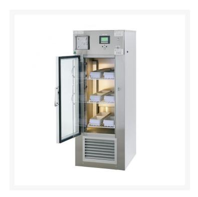
Arrowsmith and Grant AG36BP Glass Door Blood Refrigerator is a single glass door upright vertical fridge, has an external dimension of 555mm (W) x 725mm (D) x 1520mm (H), 200 litres of storage capacity, temperature range of 2.5 to 5.5 degrees centigrade, and automatic defrost.
