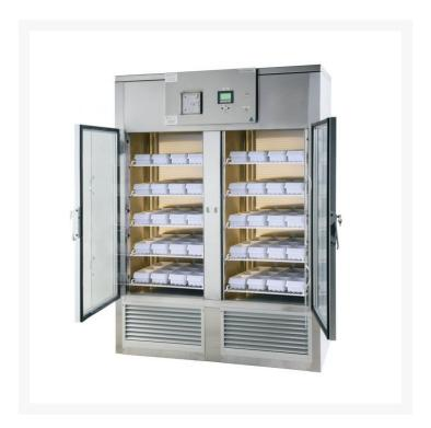
Arrowsmith and Grant AG224BP Glass Door Blood Refrigerator has a dimension of 1475mm (W)  $\times$  805mm (D)  $\times$  2000mm (H), can hold 520  $\times$  450ml of blood packs 1050 litres, temperature range 2.5 to 5.5 degrees centigrade, and refrigerant gas R507.
