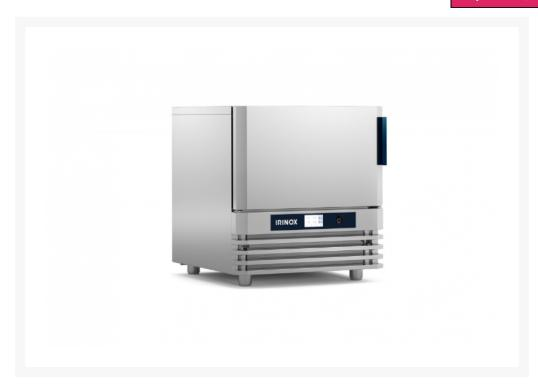
IRINOX-MF-NEXT-S-TURBO has a increase yield per cycle 18kg (chill) & 15kg (freeze) in its performance, it also has essential and excellence configurations, 90 to -18 centigrade temperature scale, climate class of 5, runs on R452A gas, USB connection for downloading HACCP data, ultra-compact entry level reach in GN 1/1 blast chiller and shock freezer offering powerful food production gains on a small footprint.
