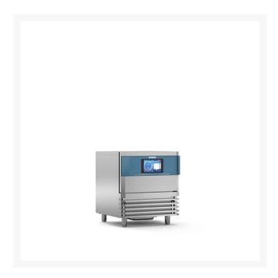
IRINOX-MF-NEXT-S-ECO has a standard performance but with very little noise output, it has 2 configurations: essential and excellence, it has a variety of tray capacities you can choose depending on how you use it, a temperature scale of 90 to -18 degrees centigrade, an ambient temperature of 32 centigrade, 0.97kW energy absorption, R290 gas, easy to adapt interface.
