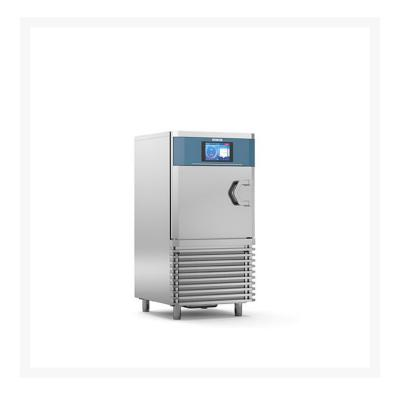
IRINOX-MF-NEXT-M-TURBO owns a boosted yield of 65kg on quick freezing cycle, temperature span of 90 to -18 degrees centigrade, ambient rating of 40 degrees, power absorption of 5.4kW, also works on R290 gas, adaptable interface, HACCP data backup, variations of tray capacities: 9(GN1/1 or 600x400), 12(GN1/1 or 600x400), 18GN1/1 or 600x400).
