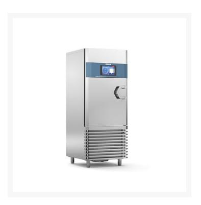
IRINOX-MF-NEXT-L-TS has increased performance in cooling and freezing while having a very low level of noise emission. Maximum power consumption is 8.3kW, operates on R290 gas, has a range of tray capacities such as 27(GN1/1 or 600x400), 18(GN1/1 or 600x400), and 13(GN1/1 or 600x400). 90 to -18 degrees centigrade temperature scale and climate class of 5.
