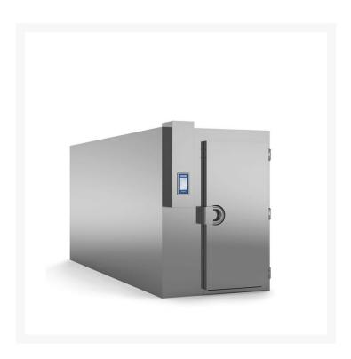
Irinox-MF-750.2-4T has a design of sunken floor, knockdown, and pass-thru. It can yield 750kgs of ice per shock freeze cycle, it has an energy absorption of 9.4kW/h, also has a temperature range of 90 to -18 degrees centigrade, and an ambient temperature of 32 degrees centigrade, and have 2 different tray capacities such as 8x20(GN 1/1) and 4x20(GN 2/1).
