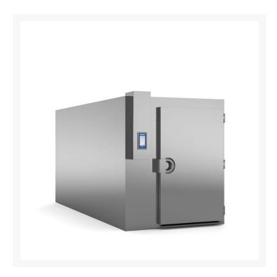
Irinox-MF-500.2-3T-LARGE has 500 kilograms of ice yield per cycle, it has a temperature range of 90 to -18 degrees centigrade, its different tray capacities are 12x20(GN 1/1), 6x20(GN 2/1), 9x20(400x600mm), 4x20(800x600mm), and 3x20(1000x1000mm). It has 7.1kW/h energy consumption, it also runs with R452A refrigerant. This has a sunken floor and pass-thru design, it also has a larger usable area.
