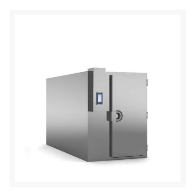
Irinox-MF-350.2-3T has an ice production of 350 kilograms, its max energy consumption is 7.7kW/h, an eco-friendly R452A refrigerant gas, a temperature range of 90 to - 18 degrees centigrade, with an ambient temperature of 32 degrees centigrade, a HACCP software, and different type of tray capacities like  $6\times20(GN 1/1)$ ,  $3\times20(GN 2/1)$ ,  $6\times20(400\times600)$ , and  $3\times20(800\times600)$ .
