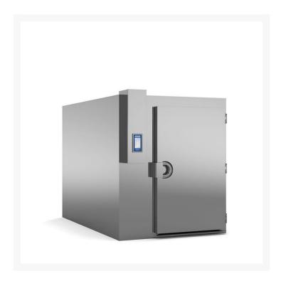
Irinox-MF-350.2-2T-LARGE has a shock freezing cycle yield of 350kg of ice in 90 to -18 degrees centigrade, an R452A refrigerant gas, a HACCP control protocol, a 32 centigrade ambient temperature, a 4.7kW/h power consumption, and a variety of tray capacity like 8x20(GN 1/1), 4x20(GN 2/1), 6x20(400x600), 3x20(800x600), and 2x20(1000x1000).
