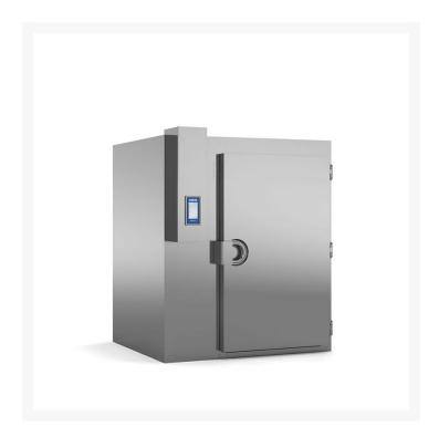
Irinox-MF-180.2 LARGE has a larger capacity and a sunken floor version, it has a different capacity of 4x20(GN 1/1), 2x20(GN 2/1), 3x20(400x600), 1x20(800x600), and 1x20(1000x1000). It also has HACCP protocol software, can make 180 kilos of ice in a temperature range of 90 to -18 centigrade, with 32 degrees centigrade ambient rating, a 2.4kW/h energy consumption, and R452A refrigerant gas.
