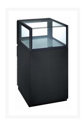
Anvil DSD0001 Single Drawer Showcase is constructed with a black brushed 304 stainless steel body and a Triple glazed ITO safety glass with a heater. The maximum loading height of the drawer is 300mm and the rear sliding drawer with illuminated base. Extended gold star warranty 2 years parts + 1-year labor.
