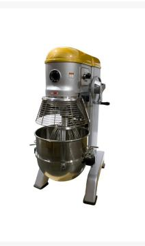
Anvil PMA1060 60 Quart Gear Driven Planetary Mixer has four different speeds 84rpm, 148rpm, 248rpm, 436rpm. The other features include 3HP air cooled motor, direct drive gear driven transmission, long life gear box, grease packed ball bearing, and comes with whisk, hook, paddle, and additional bowl dolly.
