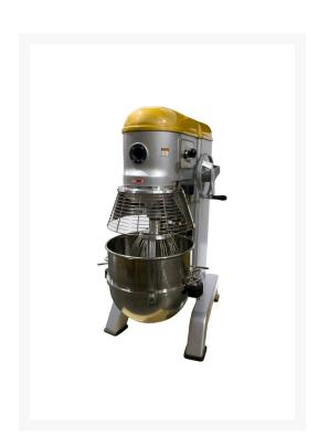
Anvil PMA1060 60 Quart Gear Driven Planetary Mixer has four different speeds 84rpm, 148rpm, 248rpm, 436rpm. The other features include 3HP air cooled motor, direct drive gear driven transmission, long life gear box, grease packed ball bearing, and comes with whisk, hook, paddle, and additional bowl dolly.
