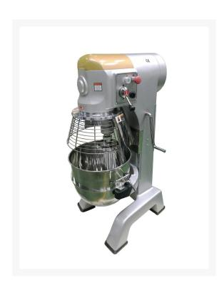
Anvil PMA1040 40 Quart Mixer has three different speeds 127rpm, 261rpm, 478rpm. The other features include 1.5Hp air cooled motor, direct drive gear driven transmission, long life gear box, grease packed ball bearing, and comes with whisk, hook, and paddle.
