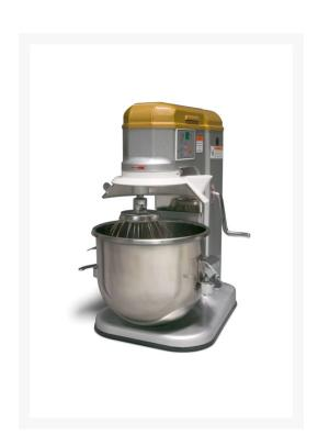
Anvil PMA1010 10 Quart Mixer has five different speeds 193rpm, 296rpm, 354rpm, 438rpm, 496rpm. The other features include 0.8Hp air cooled motor, direct drive gear driven trans, long life gear box, grease packed ball bearing, guard fitted with safety micro-switch, gears and shafts made of heat treated alloy steel.
