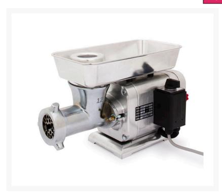
Anvil MGT3012 Heavy Duty Meat Mincer has vast capacity of 200kg per hour and supplied with sausage filler tunnel, suasage filler spacer, with 3.1mm, 4.5mm, 6mm and 9mm plates, and 4 knives. Additionally, it is equipped with forward and reverse functions.
