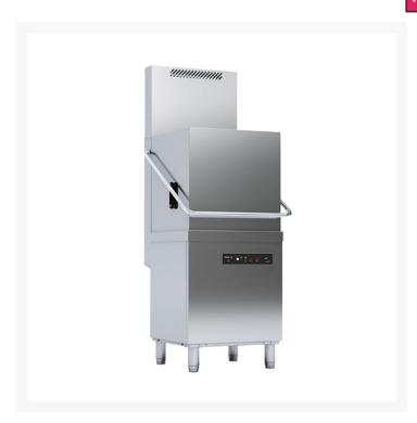
EVO-CONCEPT pass-through dishwasher with drain pump and detergent dispenserHourly production: 60 baskets/hour - 720 dishes/hour. Clearance (max ware height): 440m. Wash cycles: 55-75-120 seconds. Double rotating wash and rinse systems, made of AISI-304 stainless steel. Water consumption: 2.4 litres/rinseSafety magnetic switch for hood opening. Adjustable legsSupplied with 1 base basket; 1 plate basket and 2 cutlery containers. WaterMark approved
