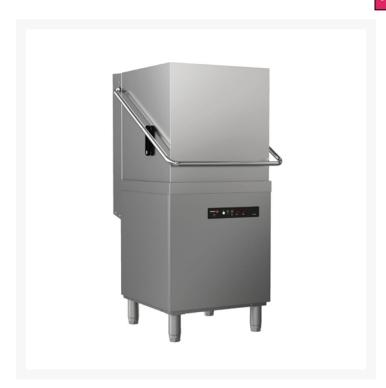
EVO-CONCEPT pass-through dishwasher with drain pump and detergent dispenser. Hourly production: 60 baskets/hour - 720 dishes/hour. Clearance (max ware height): 440mm. Wash cycles: 55-75-120 seconds. Double rotating wash and rinse systems, made of AlSI-304 stainless steel. Water consumption: 2.4 litres/rinse. Safety magnetic switch for hood opening. Adjustable legsSupplied with 1 base basket; 1 plate basket and 2 cutlery containers. WaterMark approved
