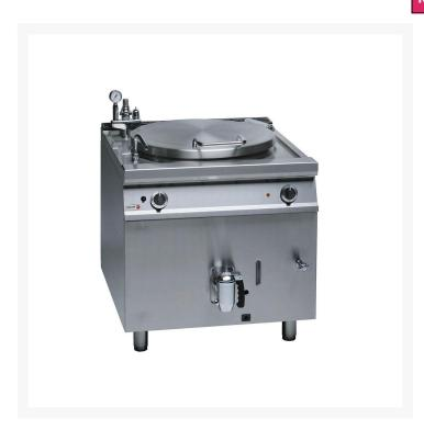
Tank: 600mm? x 500mm H Volume: 150LNG or LPGSurface tops manufactured in 2mm thick AISI-304 stainless steelLaser-cut joints, automatic welding and polishes. Screws hidden from viewDouble walled lid balanced by means of a hinge with front handle, with diagonal opening to 75° which allows the lid to be kept open in any positionWell stamped into the surface top by robotic welding, manufactured in 304 S/S, with the bottom of the well in AISI-316L stainless steel.
