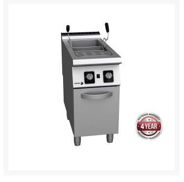
Grill x 1Size: GN-1/1NG or LPGSurface tops manufactured in 2mm thick 304 stainless steelStandard configuration: three 1/3 type baskets per tankDraining of tank by means of high temperature resistant mechanical ball valve with safety overflowAutomatic safety system that breaks the circuit if the water runs outControls set on a protective base with a system against water infiltrationAccess the components from the front
