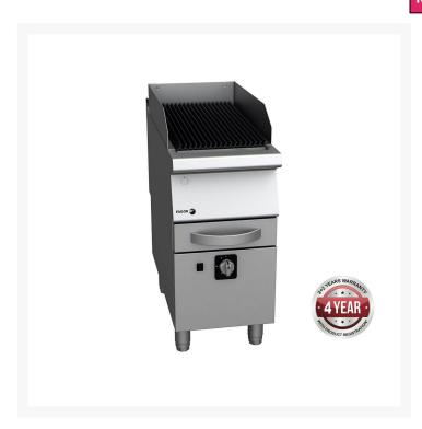
NG or LPGSurface tops manufactured in 2mm thick 304 stainless steelReach a high temperature (400°C)The iron grills are reversible, with different finishes on each sideGrid area: 1Total power: 11KW
