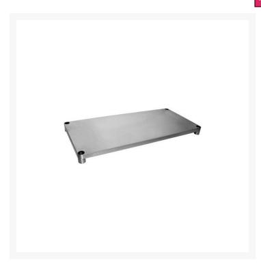
SUS7-2400/A Solid Undershelf constructed with 1.2mm thick SUS304 (18/8) grade with hairline finish. Special U channel reinforcements under to suit the bench type & size. Special U channel reinforcements to match the bench type & size, and the U channel width increases as the bench size rises.
