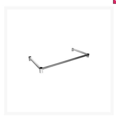
LB7-2400/A Leg Brace is stainless steel commercial leg brace with 1.2mm SUS304 (18/8) and BA finish. Comes with 38 diameter 1.2 mm tube. It measures 490mm wide x 590mm deep. Leg brace must be used for stability when no undershelf is required.
