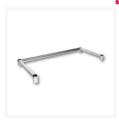
LB6-0600/A Leg Brace is stainless steel commercial leg brace with 1.2mm thick SUS304 (18/8) grade stainless steel and BA finish. Comes with 38 diameter 1.2mm tube. It measures 490mm wide x 590mm deep. Leg brace must be used for stability when no undershelf is required.
