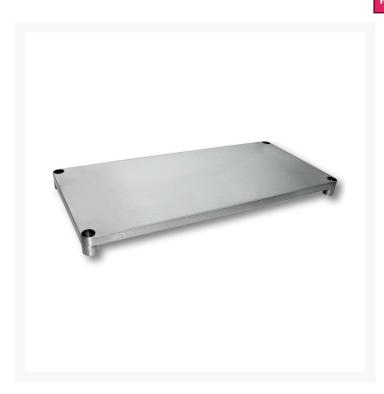
SUS6-2100/A Solid Undershelf comes with 1.2mm thick SUS304 grade stainless steel with a hairline finish for storage addition to a commercial workbench. Special U channel reinforcements under to suit the bench type & size. Width of U channel increases with the bench size.
