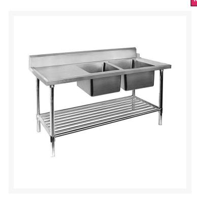
Right Inlet Double Sink Dishwasher Bench DSBD7-1800R/A for commercial kitchen and hospitality workspace. Stainless steel-backed 180mm high; 30mm thick splashback protects the area behind the sink from spilling. Two right positioned bowls, Legs with fully adjustable S/S polished disc feet. SUS304 (18/8) grade benchtop with U channel reinforcements.
