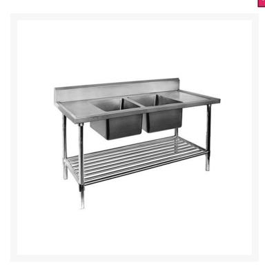
Double Centre Sink Bench with Pot Undershelf DSB6-1800C/A is durable and a great addition to your open commercial kitchen. Comes with centre bowl positioning, fully welded bowls, 15mm wet edge. 1.2mm thick pot undershelf with stainless steel backed splashback 150mm high, 30mm thick. Benchtop lined with 15mm thick XPS board and stainless steel panel. 90mm diameter drain hole.
