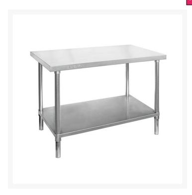
WB7-1200/A Stainless Steel Workbench with adjustable solid undershelf. Comes with 1.2mm thick SUS304 built benchtop lined with 20mm thick XPS board & S/S panel. Special U channel reinforcements under benchtop and undershelf. 1.2mm thick legs with fully adjustable S/S finished disc feet with lockable castor kits and optional drawers available.
