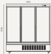
Gross volume: 1665 LExterior dimensions in mm:  $1875w \times 740d \times 2100h$ Number of adjustable shelves: 15 Temperature set range: 0°C to +10°C Gross/net weight: 284/245 kg Energy consumption in **24h**: 8.28 kWh
