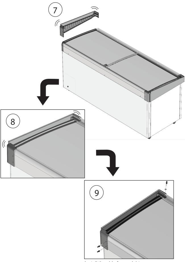
Install the side frame right and secure by screw.
