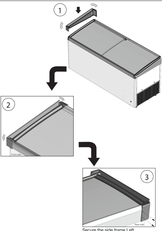
Secure the side frame Left by screw (Self drilling #8) tighten completely by powered screwdriver.
